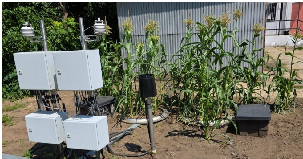
Figure 6. Experimental setup of the sweet corn lysimeter trial and crop stand at the early growth stage
